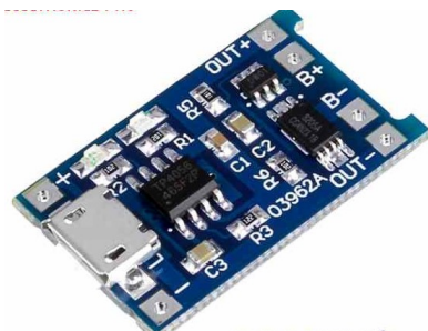
Figure 12: Battery Charging Module
