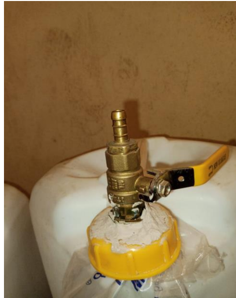
Plate 1: Digester with flammable biogas Plate 2: Gas outlet with no black traces (H 2 S)
