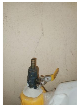
Plate 7: Digester with non- flammable biogas; Plate 8: Gas outlet with black traces (H 2 S)
