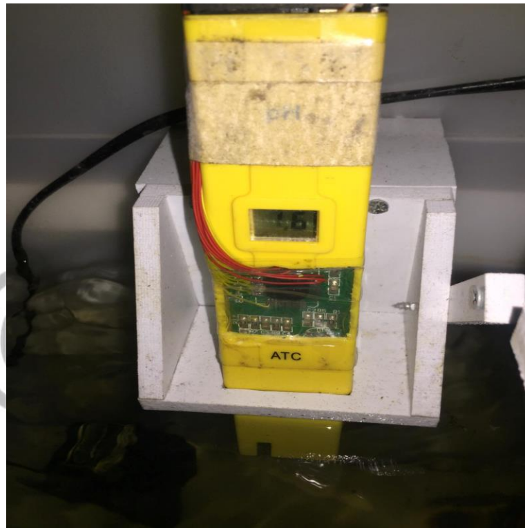
Figure 4.12. pH level sensor floating in the water to get data
