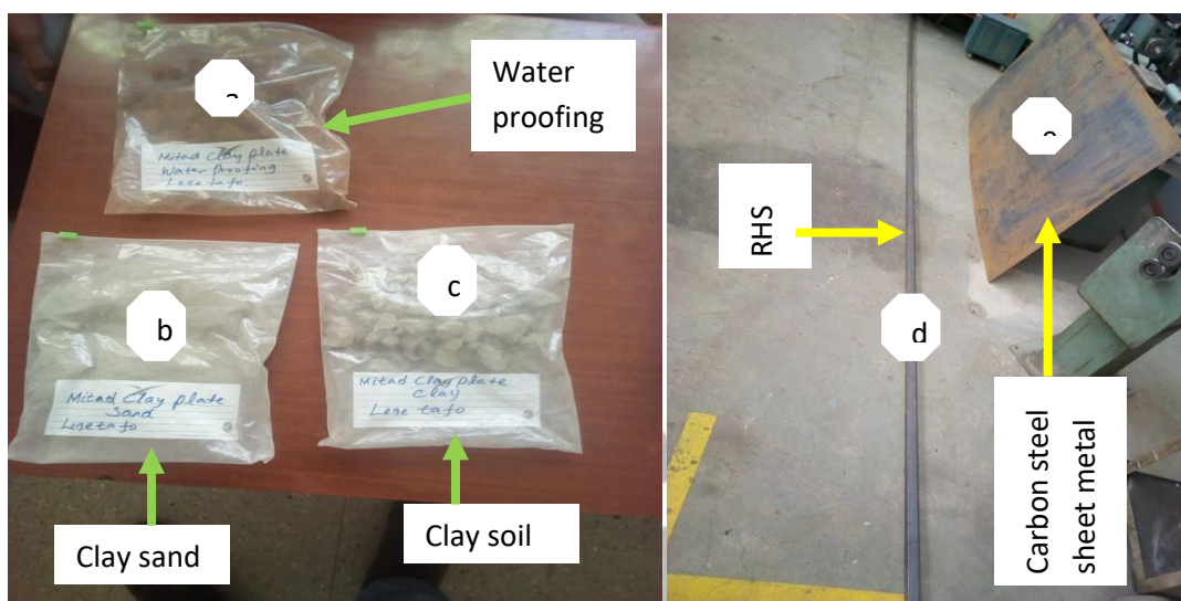
Figure 2 shows raw materials: a) waterproofing, b) clay sand, c) clay soil, d) RHS, and e) carbon steel sheet metal for developing prototype.
