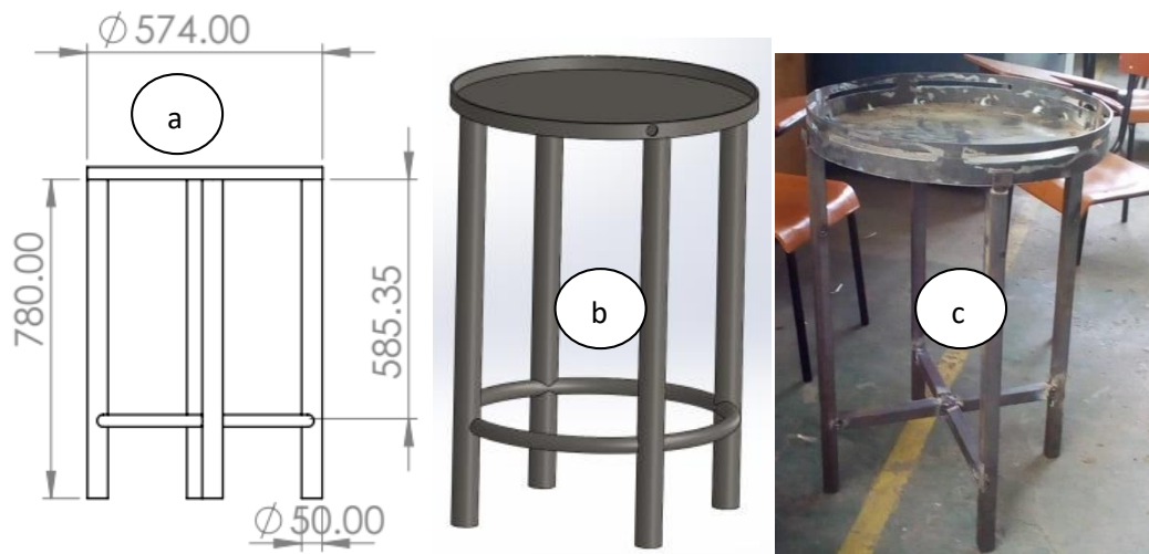
Figure 4 of support stands a) views, 3-D solid work model, and c) manufactured
