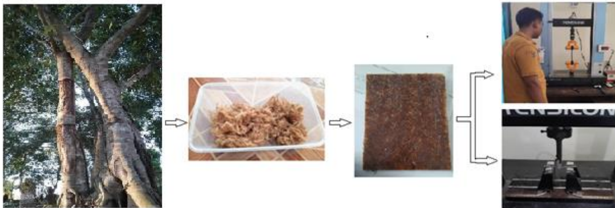
Figure 1 Fiber preparation, fabrication, tensile and bending testing of composites.
