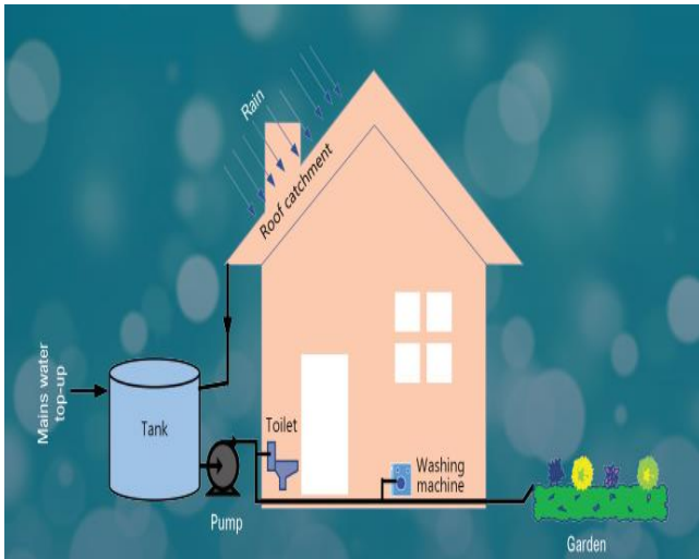
Fig 1.0 Ashok et al (2019) Showing the various uses of rainwater in an urban setting (Ashok K. Sharma, Donald Begbie and Ted Gardner. Rainwater Tank Systems for Urban Water Supply IWA Publishing 2019
