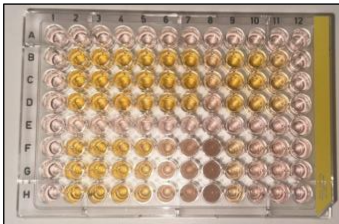
Figure 22 - Color change upon dissolution of formazan salt indicates cell viability from mitochondrial activity
