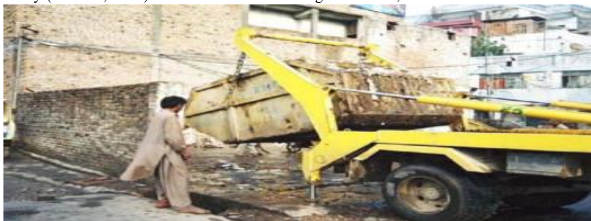
Figure 1 View of 5 m 3 container that is being lifted mechanically by Mazda arm roll.
