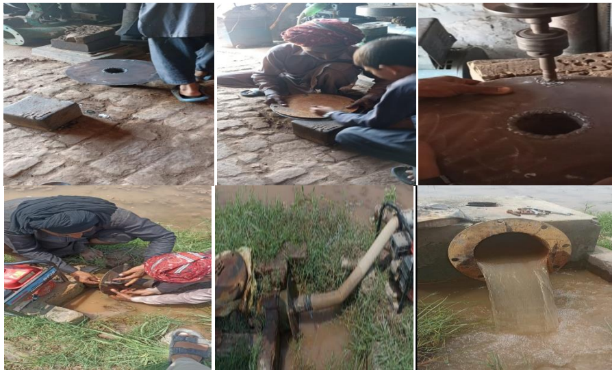
Pictorial view showing the long neck weld flange plate (LNWFP) technology used in precision agriculture to uplift rain water harvest from paddy field having excessive water
