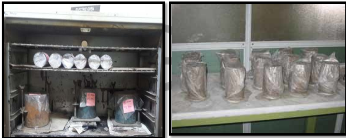
Figure 1 and Figure 2: Curing arrangements for sealed samples
