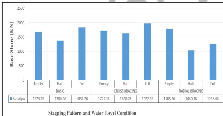
Figure 7: Comparison of Base Share v/s different staging patterns and water level under fixed-based condition
