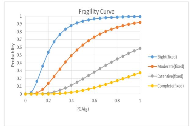
Figure 12: Fragility curve for half full case of fixed based condition
