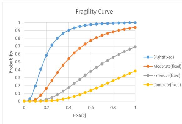
Figure 11: Fragility curve for half full case of fixed based condition
