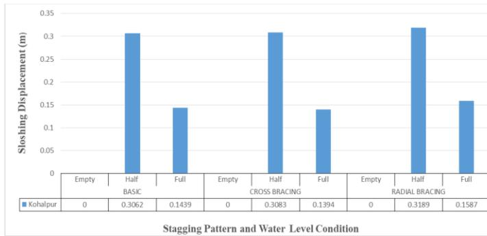
Figure 6: Comparison of Sloshing Displacement v/s different staging patterns and water level under fixed-based condition
