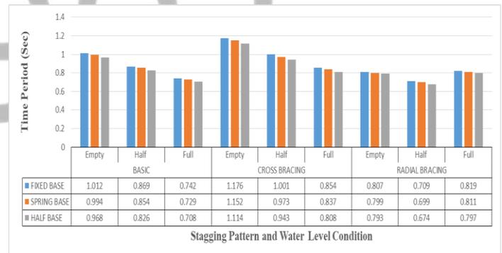
Figure 9: Comparison of time period v/s different staging patterns and water level under different base condition
