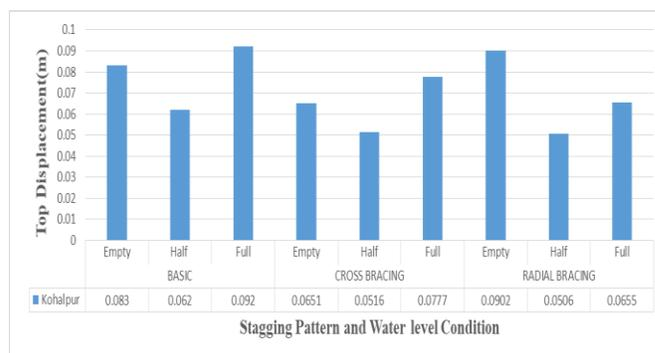
Figure 4: Comparison of Top Displacement v/s different staging patterns and water level under fixed based condition
