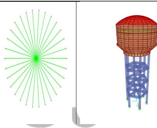
Figure 2: Spring Mass Model of Tank
