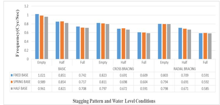
Figure 8: Comparison of Frequency v/s different staging patterns and water level under different base conditions
