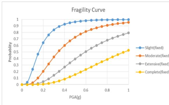
Figure 10: Fragility curve for full case of fixed based condition
