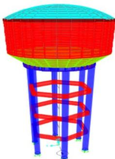
Figure 3: FE model of elevated water tank with basic type
