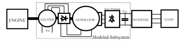
Block diagram of the synchronous generation system [5]
