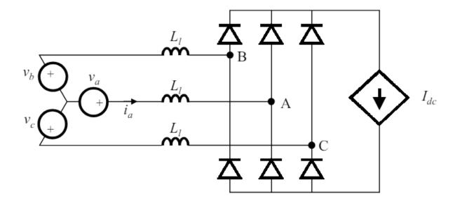
The real time voltage source feeding on current source dc load through a diode rectifier
