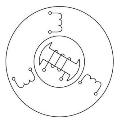
Two-pole Synchronous Machine [5]
