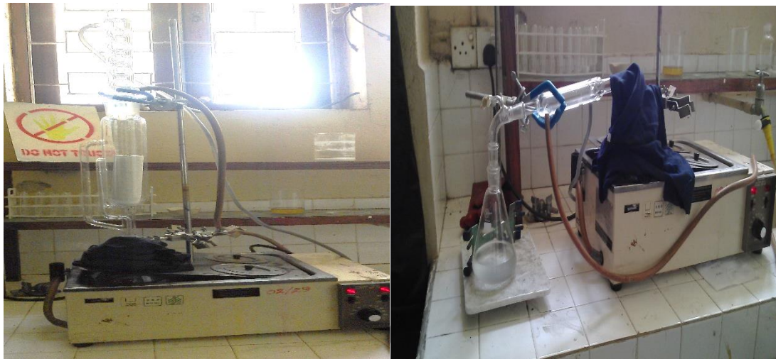
Figure 9. Soxhlet apparatus & hexane vaporization process
