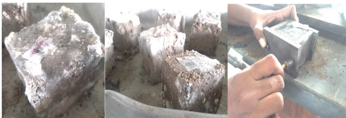
Figure 6.Fungus attack and demolding process
