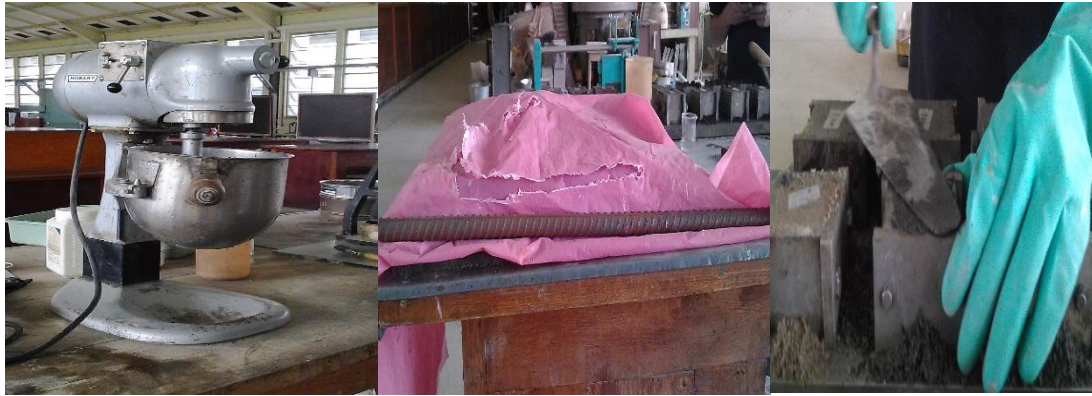
Figure 2. Mixing bowl, moist-air cabinet & tile preparation
